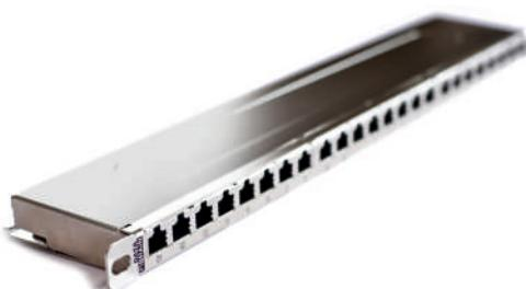
FIBRAIN DATA shielded patchpanels Express series are complied to requirements of category 5e (class D). Such connections support majority of contemporary applications. They are equipped with special 9 pin angle connectors IDC-LSA providing ease and fast installation. Such kind of connector provides high transmission parameters and resistance to interference.
