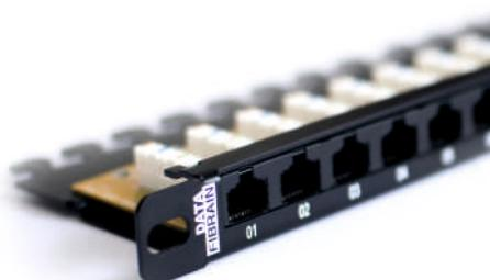
FIBRAIN DATA Unshielded patchpanels Quick series fully comply with requirements of cat. 6 (Class E) and perform transmission of 250 MHz. They are equipped with angled connectors IDC-LSA which ensure ease and rapidity of assembly. Additionally has shelf in L-shape design which allows to make easy changes, extension, reconfiguration. Easy access to IDC connectors allows maintenance and changes in connections.
